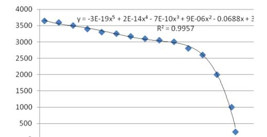
Figure 2: C130 Range (nm) as a function of load
